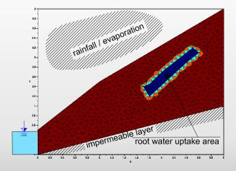
Mathematical modeling of water dynamics in soils - a tool for smart management of irrigation networks.
